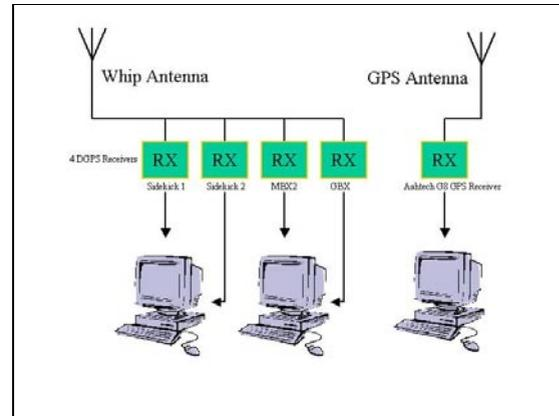
**Fig. 7: Experimental set-up for testing RAAS concept**
