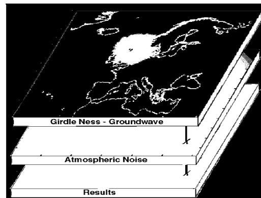
**Fig. 2: New software architecture employs a three-dimensional array. This simple example has just three layers. They hold the groundwave strength of a single beacon, the atmospheric noise, and (in the results layer) coverage computed using the first two.**
