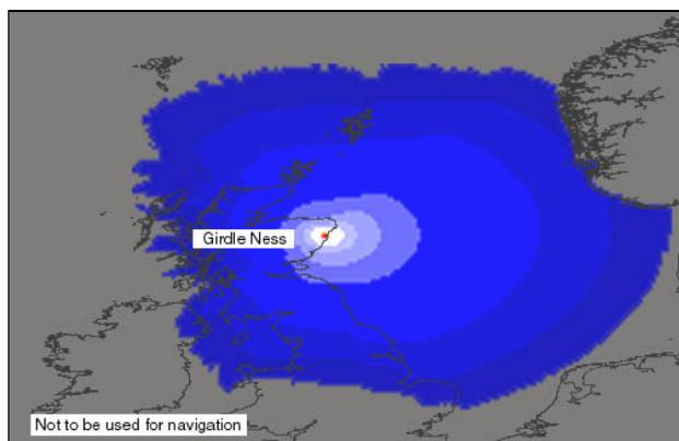
**Fig. 3: Groundwave field strength contours of a beacon at Girdle Ness, Scotland. The outer boundary is the limit of daytime interference-free coverage computed using data from top two layers in Fig. 2.**
