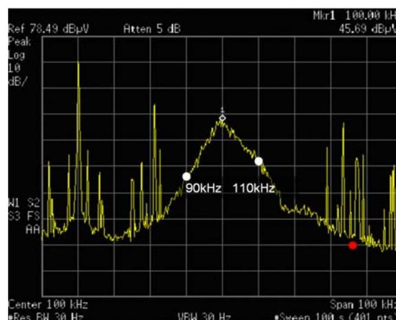
**Figure 4: Spectrum from 50kHz-150kHz at 33km from Anthorn**
