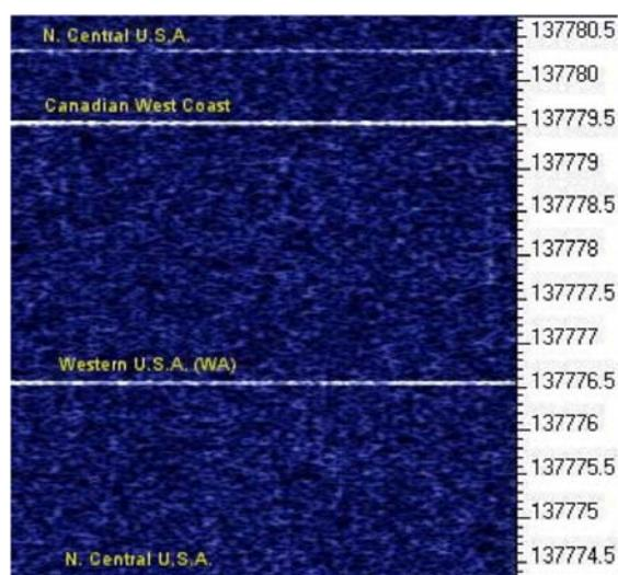
**Figure 11: US Loran spectral lines (from [4])**
