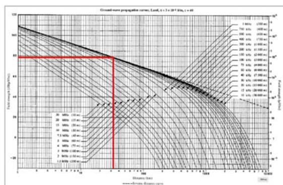
**Figure 9: Groundwave propagation curves (from [2])**
