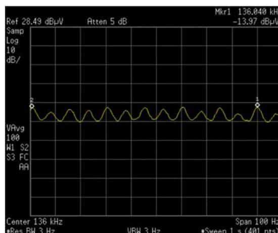
**Figure 7: 100Hz-wide spectrum around 136kHz at 33km from Anthorn**
