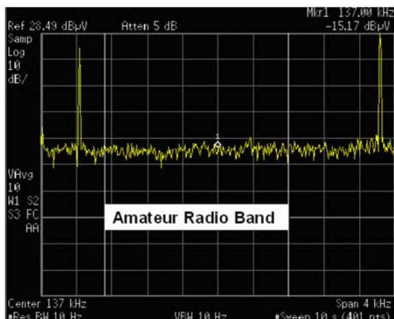
**Figure 5: Spectrum from 135kHz-139kHz at 33km from Anthorn**
