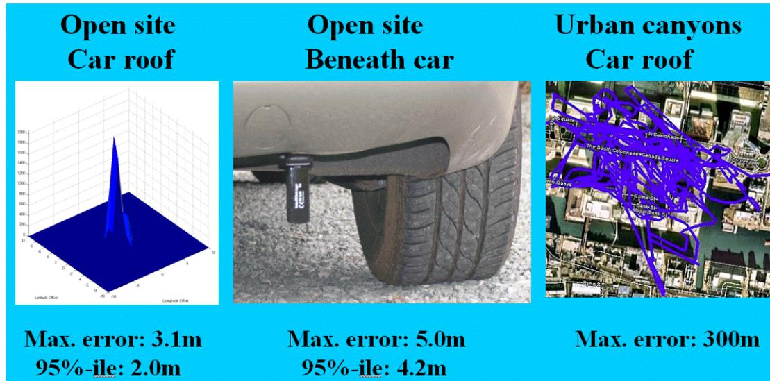
**Figure 5: Examples of GPS accuracy**
