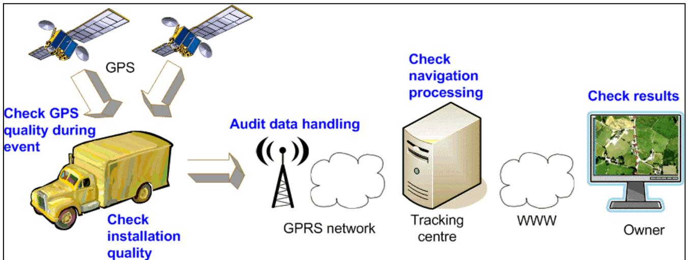
**Figure 3: Vehicle tracking system with checks (in blue) to establish quality of evidence**
